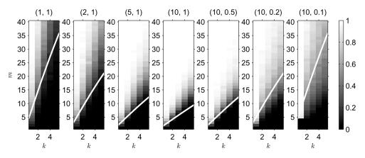
Fig. 1. Simulated success probability of ML detection for n = 20 and many values of k, m, SNR, and MAR. Each subgraph gives simulation results for  $k \in \{1, 2, ..., 5\}$  and  $m \in \{1, 2, ..., 40\}$  for one (SNR, MAR) pair. Each subgraph heading gives (SNR, MAR). Each point represents at least 500 independent trials. Overlaid on the intensity plots is a white curve representing (14).
