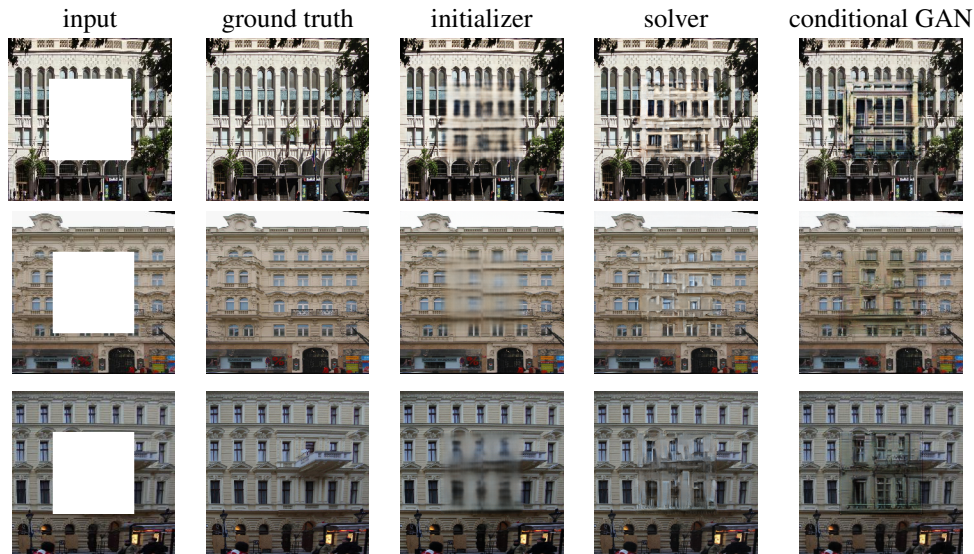
Figure 11.24: Pattern completion by conditional learning. Each row displays one example. The first image is the testing image ( 256 \times 256 pixels) with a hole of 128 \times 128 that needs to be recovered, the second image shows the ground truth, the third image shows the result recovered by the initializer (i.e., conditional generator model), the fourth image shows the result recovered by the solver (i.e., the MCMC sampler of the conditional energy-based model, initialized from the result of the initializer), and the last image shows the result recovered by the conditional GAN as a comparison.
