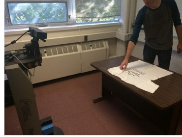
Figure 1: The setting of our situated task learning where a human teacher teaches the robot how to fold a T-shirt through both task demonstrations and language instructions.
