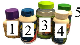
Fig. 3: Bottles used in experiments with different safety mechanism: (1) push-and-twist , (2) pinch-and-twist , (3) push-and-twist , and (4) push-and-twist . (5) Bottle with no safety mechanism.
