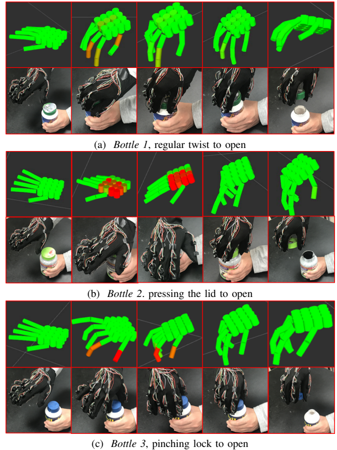
Fig. 11: Action sequences and visualizations of opening three types of bottles
