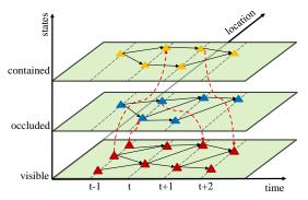
Figure 5. Transition graph utilized to formulate the integer linear programming. Each node m has its location  $l_m$ , state  $s_m$ , and time instant  $t_m$ . Black solid arrows indicate the possible transitions in the same state. Red dashed arrows indicate the possible transitions between different states.
