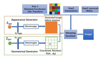
*Figure 1.* An illustration of the proposed model. The model contains two generator networks: one appearance generator and one geometric generator. The two generators are connected with a warping function to produce the final image. The warping function includes a geometric transformation operation for image coordinates and a differentiable interpolation operation. The refining operation is optional for improving the warping function.
