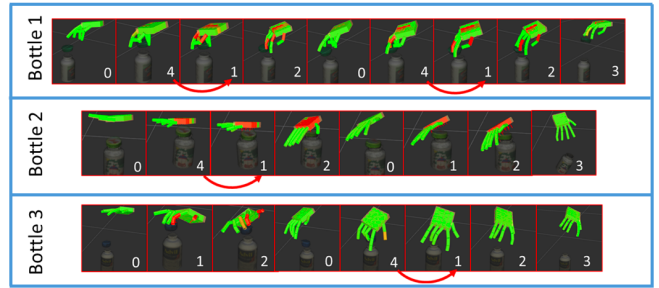
Fig. 6: Key frames of opening various bottles with T-AOG. The numbers indicate the cluster labels and the red arrows indicate the merges triggered by the parsing of T-AOG.
