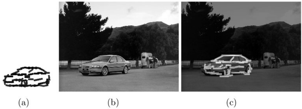
Fig. 14 Experiment 2.1. (a) Template learned from training images in Experiment 1.1. h() is the sigmoid transformation. Size of template is 82 \times 164 . (b) Testing image. The inference algorithm is run over 15 resolutions, from 50 \times 67 to 751 \times 1001 . (c) Superposed with sketch of the 60 elements of the deformed active basis at the optimal resolution and location
