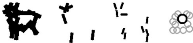
Fig. 51 Experiment 9.1. The selected Gabor elements (illustrated by bars) at 3 different scales and the selected DoG elements (illustrated by circles, and larger circles are darker than smaller ones). The lengths of the Gabor elements are 35, 25, and 17 pixels respectively. The sizes of the DoG elements are 77 and 55 respectively. The allowed activity of location is 4 pixels for both Gabor and DoG elements
