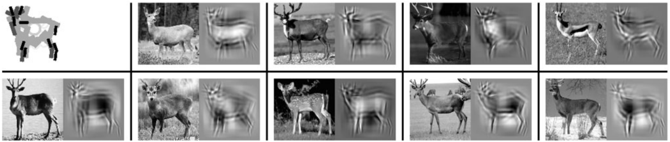
Fig. 52 Experiment 9.1. The first block displays all the 50 selected Gabor and DoG elements. The smaller Gabors are illustrated by darker bars . The remaining blocks display the original images and the corresponding reconstructed images. The image size is 102 \times 100
