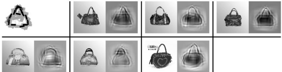
Fig. 57 Experiment 9.5. The first block displays all the 50 selected Gabor and DoG elements. The remaining blocks display the original 100 \times 100 images and the corresponding reconstructed images
