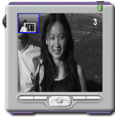
Figure 19: A tour over a Gaussian pyramid. Visiting the decomposed quad-tree nodes in a sketch pyramid is an efficient way to automatically convey a large image’s informational content.
