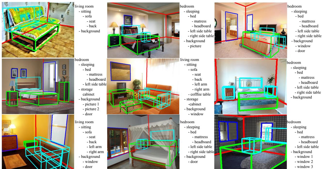
**Fig. 17** Parsing results include cubic objects (green cuboids are detected by bottom-up step, and cyan cuboids are detected by top-down prediction), planar objects (blue rectangles), background layout (red box). The parse tree is shown to the right of each image.
