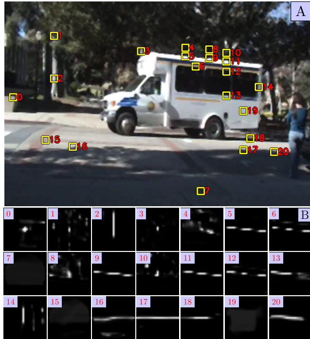
Fig. 3 Posterior probability map of SSD model — (A) patches with numbers; (B) probability map of each numbered patch. Better viewed in color.
