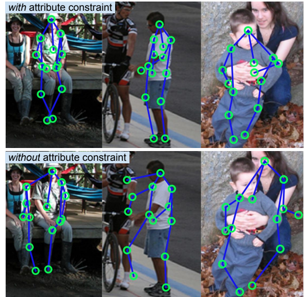
Fig. 3. Attribute constraints. We infer the pose pg^* either using Equation 18 or 20. When we do not have attribute constraints (i.e. using Equation 18) the model selects the part that maximize the scores in local, and the part could come from different person, when there are multiple people close. However, by having the attribute as global constraints (i.e. using Equation 20), we can enforce model to have consistent attributes which subsequently results in better pose-estimation.
