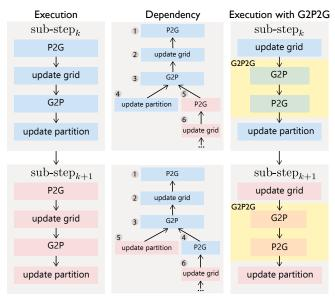
Fig. 4. **MPM pipeline reformulation**. The left column shows the traditional MPM pipeline, and the middle one illustrates an analysis of data dependencies among the sub-steps. The exchange of the *update partition* at the current time step k and the P2G at the next time step k + 1 would not break the data dependency or the execution correctness, making it possible to reorder and assemble the G2P and the P2G to form a more efficient G2P2G kernel, as shown on the right.
