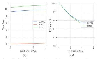
Fig. 12. **Weak scaling; compact layout.** (a) The per time-step wall time remains steady with an increasing number of GPUs for the *G2P2G* and overall performances. The additional overhead of halo tagging is growing but remains insignificant. (b) Both the *G2P2G* kernel and the overall efficiencies still stay around 95% even when employing 4 GPU devices.
