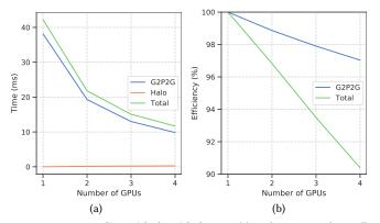
Fig. 14. **Strong scaling; side-by-side layout.** (a) Both *G2P2G* and overall performances scale well with an increased number of GPUs. The additional overhead of halo tagging is growing but remains insignificant. (b) The loss of the strong scaling of *G2P2G* is trivial even when employing 4 GPU devices, while the overall strong scaling drops to around 90%.
