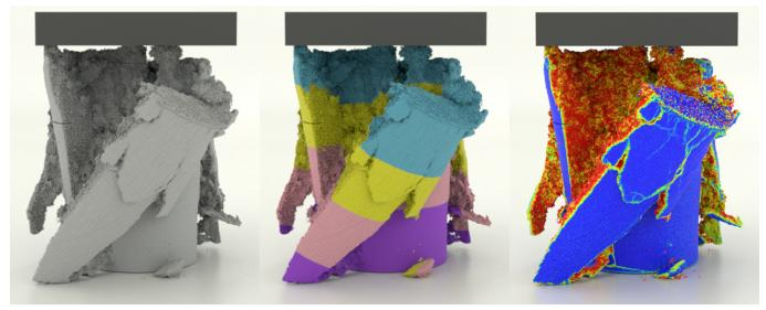
Fig. 1. **Crushing concrete**. Our system enables this concrete crushing simulation (inspired by the hydraulic press) on a single workstation with 4 NVIDIA Quadro P6000 GPUs. This simulation contains 93.8 million particles on a 1024<sup>3</sup> grid, achieving a 3.9 min/frame performance. (Left) A concrete-style render. (Middle) Coloring by GPU. (Right) Coloring by the plastic volumetric strain for visualizing the damage propagation.
