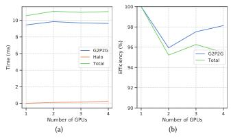
Fig. 13. **Weak scaling; side-by-side layout.** (a) The per time-step wall time remains steady with an increasing number of GPUs for the *G2P2G* and overall performances. The additional overhead of halo tagging is growing but remains insignificant. (b) Both the *G2P2G* kernel and the overall efficiencies stay above 95% even when employing 4 GPU devices.
