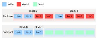
Fig. 8. Compact storage. Particles are often unequally distributed in space. Hence, uniformly allocating fixed memory space for each particle block would result in a significant amount of unused memory. Instead, a more efficient strategy is to allocate just enough particle bins for each block according to the current distribution of particles.
