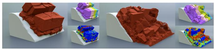
Fig. 6. Soil falling. We show a soil falling test with Non-Associated Cam-Clay (NACC) running on 4 GPUs with 53M particles and grid resolution 512×512×512. We illustrate the Multi-GPU Static Partitioning by Particles (MGSP) on the right-top corner of each subfigure. On the right-bottom corner, the NACC- $\alpha$  (the plastic volumetric strain hardening variable) is also visualized to indicate the fracture pattern, where red indicates significant material fractures.
