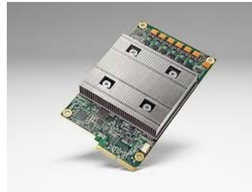
Google Tensor Processing Unit (TPU)
