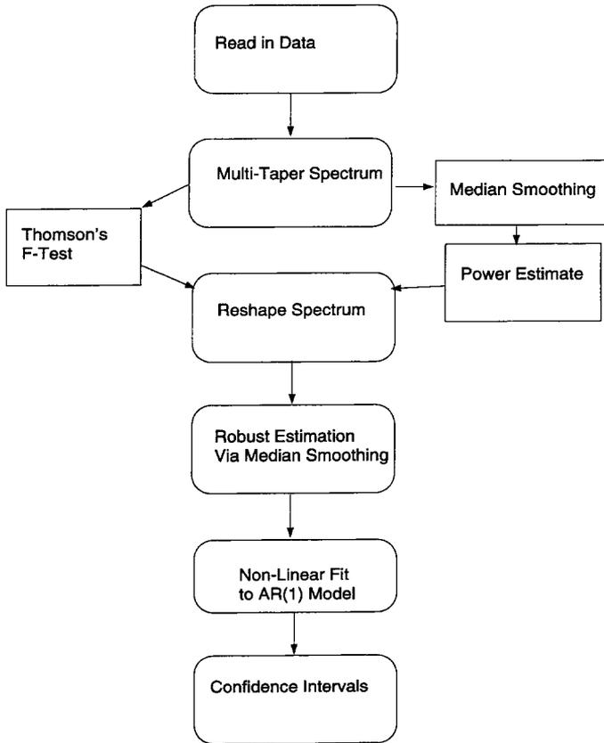
*Figure 1.* Schematic illustration of the procedure for signal identification and confidence level estimation. The reshaping step is accomplished by using a 95% or 99% confidence cut-off for both the  $F$ -test and the spectral power amplitude. Non-linear fits are calculated using Brent's method to minimize the misfit of the AR(1) model and the robust estimate of the smoothed spectrum.
