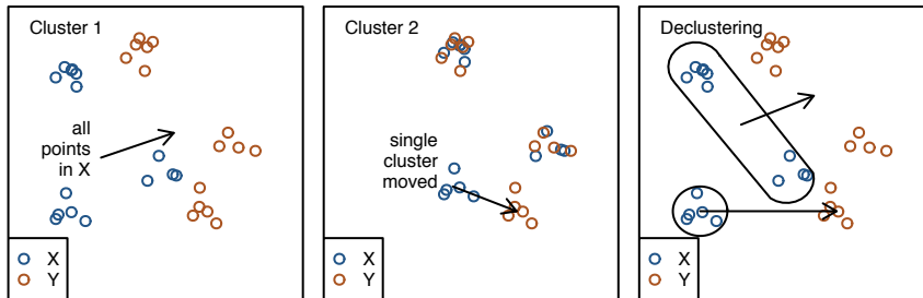
Fig. 2 The first two steps in the cluster distance are shown in the left and center panels. The right panel represents the process of removing the clustering characteristics prior to applying spike-time distance.
