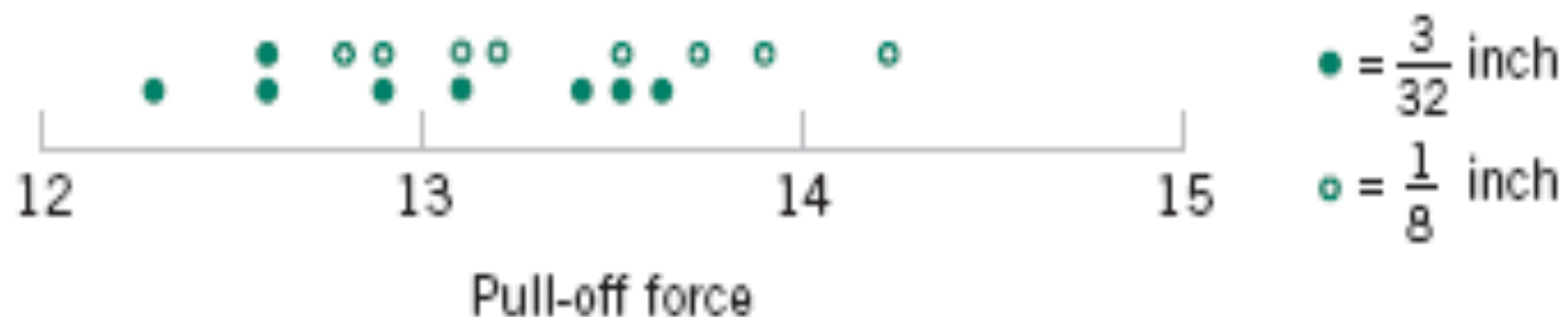
Figure 1-3 Dot diagram of pull-off force for two wall thicknesses.
