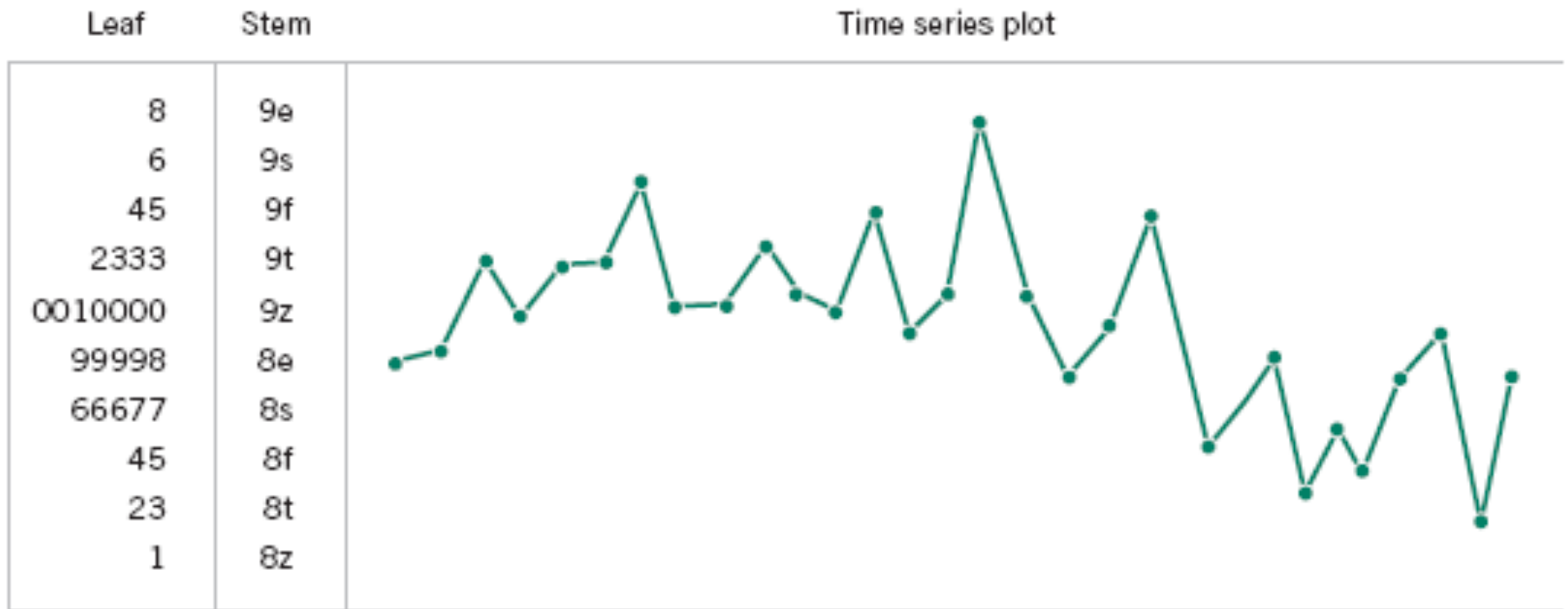
Figure 6-18 A digidot plot of chemical process concentration readings, observed hourly.
