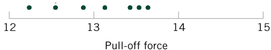
Figure 1-2 Dot diagram of the pull-off force data when wall thickness is 3/32 inch.
