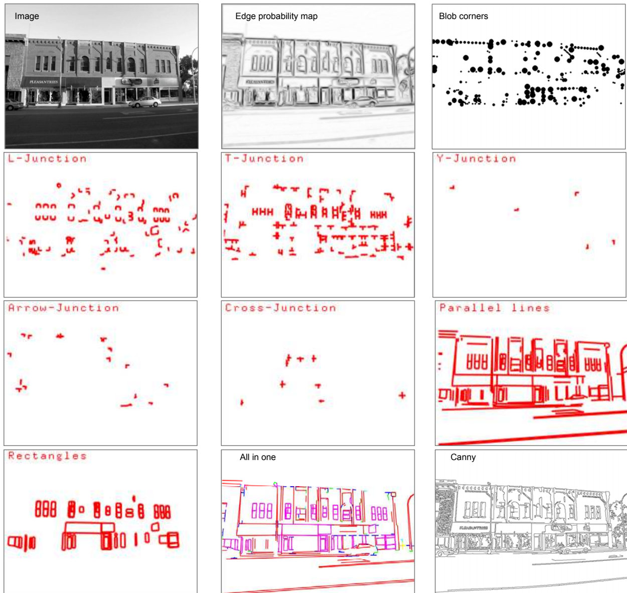
Figure 5.61: A running example of pursuing junctions and rectangles in a typical image by integrating the \alpha , \beta and \gamma processes. The left-top is the original input image. The middle-top is the edge probability map and the right-top shows the detected corners. The images in the second and the third row show the detected results of different kinds of junctions with the type name shown in the left-top in each image. The left-bottom shows the detected rectangles. The middle-bottom shows the final sketch by merging all detected results. Compared with the canny results shown in the right-bottom image, we can see that the final sketch obtained by the proposal algorithm is better. Reproduced from Ref. [168] with permission of Springer, © 2011.
