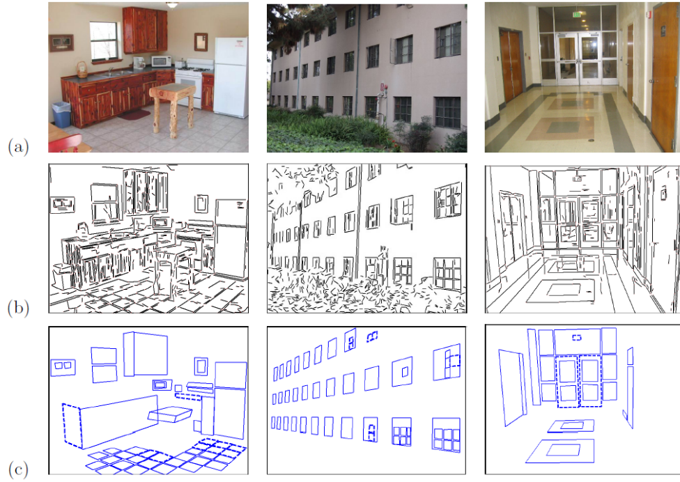
Figure 5.44: Some experimental results. (a) Input image. (b) Edge map. (c) Computed rectangle configurations and missing rectangles compared with the ground truth: true positive rectangles are shown with solid lines, false positive rectangles are shown in dotted lines and missing rectangles are shown in dashed lines. Reprinted from Ref. [62] with permission.
