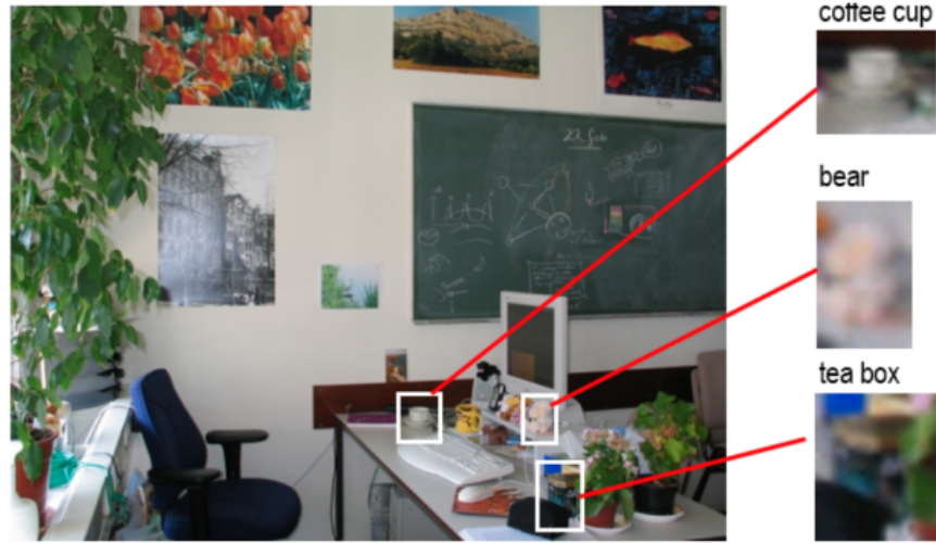
Figure 1.6: Replicating the faculty in human vision, top-down inference in computer vision can help identify unclear, e.g. , low-resolution or occluded, objects in natural images. By using the information conveyed by surrounding objects, the identities of a coffee cup, bear, and tea box in this case can be inferred.
