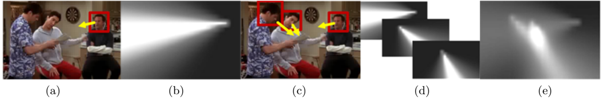
Figure 8.18: Illustration of gaze heatmap H_t^g generation procedure. With detected head position q_{t,i} (red rectangles in (a)(c)) and corresponding predicted gaze direction d_{t,i} (yellow arrows in (a)(c)), they first generate individual gaze heatmap H_{t,i}^g in (b) and (d), and then get the final gaze heatmap H_t^g in (e) via sum-pooling all the gaze heatmaps in (d). © 2018 Lifeng Fan et al. Reprinted, with permission, from Ref. [513].
