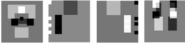
Fig. 22. The first four sparse granular features in the root node learned by the Vector Boosting algorithm and heuristic search method. They are illustrated as linear features: white blocks indicate positive granules while black ones denote negative granules. As each granule is, in fact, the average of pixels in the corresponding patch, granules of different sizes are drawn in different gray levels.
