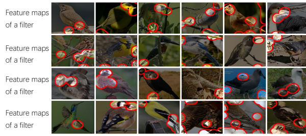
Fig. 2 Feature maps of a filter obtained using different input images (Zhang et al., 2018a). To visualize the feature map, the method propagates receptive fields of activated units in the feature map back to the image plane. In each sub-feature, the filter is activated by various part patterns in an image, which makes it difficult to understand the semantic meaning of a filter.
