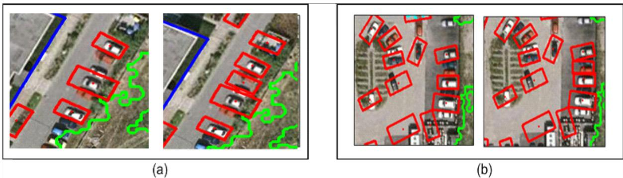
**Figure 22:** Close up views of our improvement during top-down prediction. Additional cars are added to the rows due to the presence of other collinear cars.
