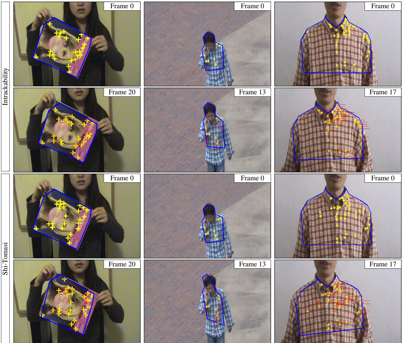
Fig. 15 Tracking comparison: In the first column, the intrackability measure tracks slightly better than Shi-Tomasi measure. In the second and third columns, the intrackability measure can distinguish subtle trackable points from the clothes, but Shi-Tomasi measure selects more repetitive feature points and makes more mismatches across frames.
