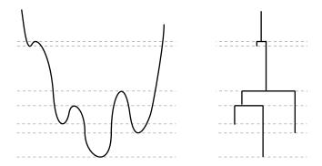
Fig. 5. Illustration of Disconnectivity Graph construction. A 1D energy landscape (left) and its associated DG (right), which encodes minima depth and the lowest known barrier between basins.
