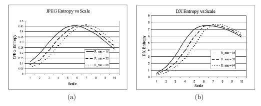
FIG. 5. The change of statistical properties versus the scale. (a) JPEG compression rate. (b) Entropy of marginal histogram of  $\nabla_x I$ .
