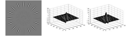
FIG. 13. (a) A sample of Gabor wavelets at different locations, scales, and orientations. (b) An example of a Gabor sine wavelet. (c) An example of a Gabor cosine wavelet.
