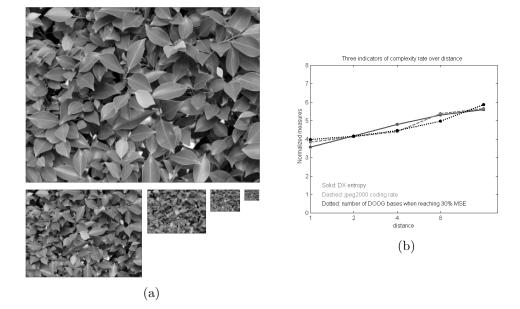
FIG. 8. (a) The original image of an ivy wall and its zoomed-out versions. (b) The change of randomness versus the zoom-out factor or equivalently the viewing distance.
