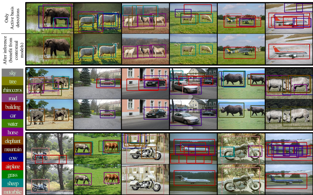
Fig. 15 Illustration of the improvement on object detections by using our framework. In each panel, the first row shows the detection results by only using the active basis model (Wu et al, 2010) (bounding boxes in different colors represent different categories) the second row show results after inference. The improvement mainly come from the advantage that our framework can integrate generative image models and the contextual models for inference.
