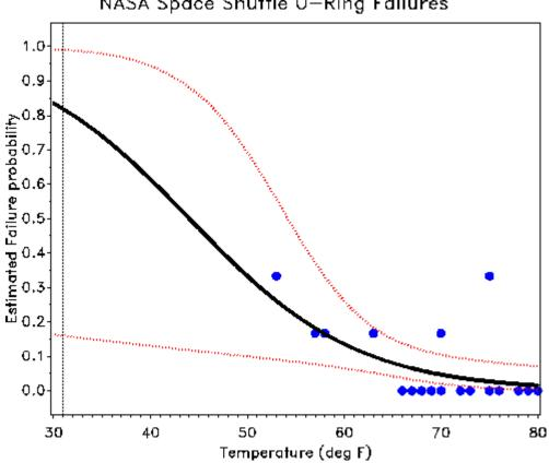
NASA Space Shuttle O-Ring Failures
