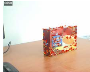
Figure 1a. A image of the coffee box and the interest points detected on its surface
