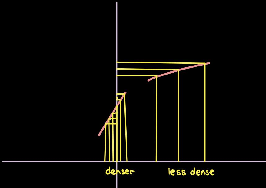
Slope controls the density of mapped points
