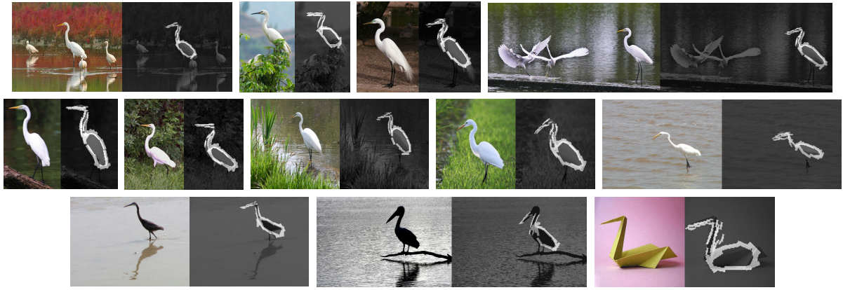
Figure 12: Detecting the objects in the testing images using the designed shape script template.
