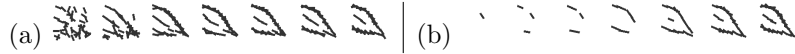
FIG. 7. (a) Template of leaf learned in the first 7 iterations of the unsupervised learning algorithm. (b) In each of iteration, the shared matching pursuit process selects wavelet elements sequentially to form each template. The sequence shows the process selecting 1, 3, 5, 10, 20, 30, 40 wavelets to form the leaf template in the last (10th) iteration.
