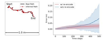
Figure 3: The learned model can perform accurate path integration. *Left*: path integration for 30 steps without re-encoding. Black: ground truth. Red: the inferred path by the learned model. *Right*: long distance (500-step) path integration error with (red) and without (blue) re-encoding by a learned 20-step RNN model over time steps. The average error and standard deviation are evaluated over 1000 trajectories.
