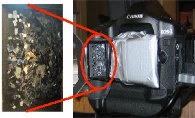
Figure 1.5: Random Lens imaging device.
