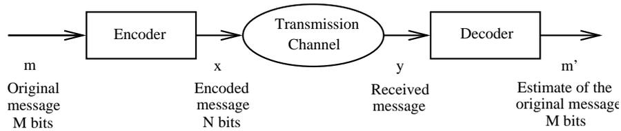
**Fig. 1.3** Typical flowchart of a communication device.
