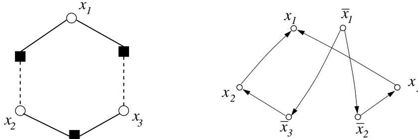
**Fig. 10.2** Factor graph representation of the 2SAT formula  $F = (x_1 \vee \bar{x}_2) \wedge (x_1 \vee \bar{x}_3) \wedge (x_2 \vee x_3)$  (left) and the corresponding directed graph  $\mathcal{D}(F)$  (right).
