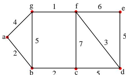
**Fig. 3.1** This graph has 7 vertices (labeled  $a$  to  $g$ ) and 10 edges. The ‘cost’ of each edge is indicated next to it. In the Minimum Spanning Tree problem, one seeks a loop-free subgraph of minimum cost connecting all vertices.
