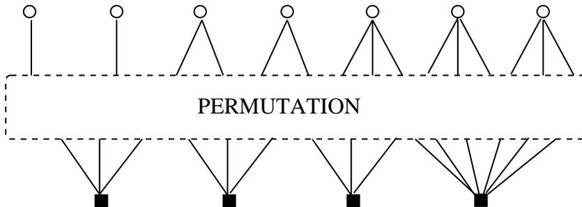
**Fig. 11.1** Construction of a graph/code with given degree profiles. Here a graph with  $N = 7$ ,  $M = 4$ ,  $\Lambda(x) = \frac{1}{7}(2x + 2x^2 + 3x^3)$ , and  $P(x) = \frac{1}{4}(3x^3 + x^6)$ . The ‘sockets’ from the variable nodes and those from the checks are connected through a uniformly random permutation.
