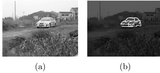
Figure 11: Experiment 2.1. (a) Testing image. The recognition algorithm is run on 10 resolutions, from 270 \times 360 to 432 \times 536 . (b) Superposed with sketch of the 60 elements of the deformed active basis at the optimal resolution 378 \times 504 . The bounding box of the template is 82 \times 164 .
