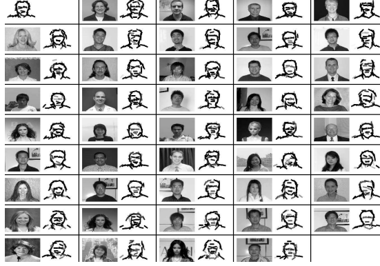
Figure 18: Experiment 3.1. Results obtained by fitting the active basis model with sigmoid transformation. The saturation level is 6. The 43 images are 127 \times 85 . The number of basis elements 40.
