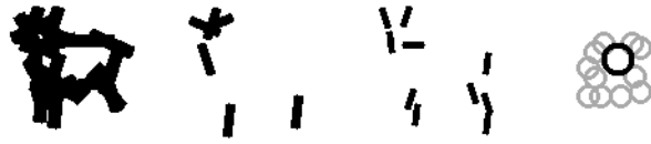
Figure 51: Experiment 9.1. The selected Gabor elements (illustrated by bars) at 3 different scales and the selected DoG elements (illustrated by circles, and larger circles are darker than smaller ones). The lengths of the Gabor elements are 35, 25, and 17 pixels respectively. The sizes of the DoG elements are 77 and 55 respectively. The allowed activity of location is 4 pixels for both Gabor and DoG elements.
