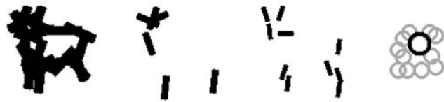
Fig. 51 Experiment 9.1. The selected Gabor elements (illustrated by bars) at 3 different scales and the selected DoG elements (illustrated by circles, and larger circles are darker than smaller ones). The lengths of the Gabor elements are 35, 25, and 17 pixels respectively. The sizes of the DoG elements are 77 and 55 respectively. The allowed activity of location is 4 pixels for both Gabor and DoG elements
