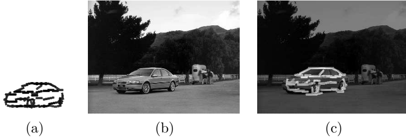
Figure 14: Experiment 2.1. (a) Template learned from training images in Experiment 1.1. h() is the sigmoid transformation. Size of template is 82 \times 164 . (b) Testing image. The inference algorithm is run over 15 resolutions, from 50 \times 67 to 751 \times 1001 . (c) Superposed with sketch of the 60 elements of the deformed active basis at the optimal resolution and location.
